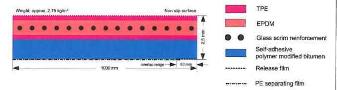
Bitumen – compatible, heat weld able, EPDM synthetic rubber membrane
